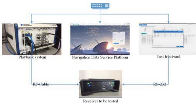
Fig. 2 Hardware framework of GNSS receiver test bench
